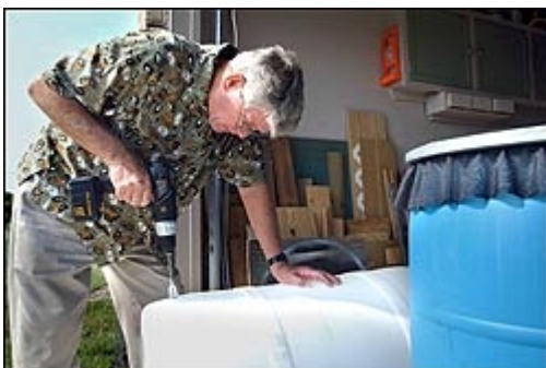
Tom Harris drills a hole in a plastic barrel to convert the container to a water-harvesting device. Tom Reel/Express-News
